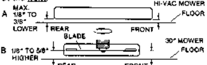
**NOTE:** Blade to floor clearance may be measured through the deck discharge opening (raise discharge deflector).
