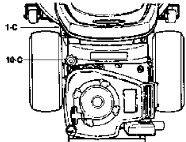
It is recommended that rear engine riders sit on the REAR BUMPER during the servicing of lubrication points on the underside. When preparing to raise the front, position BOTH hands near the center of the front frame "lip" to prevent any possibility of having fingers pinched by tie rods.
