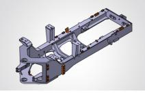
Thanks to the box-shaped structure of the rear frame side plates, the enhanced frame strength makes it easy to meet the challenge posed by harsh working conditions.
