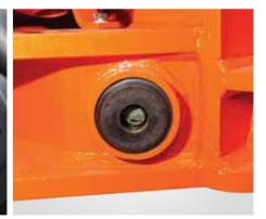
A new model of shock pad is used to provide stronger durability and reduced shock and noise, effectively relieving the driver's fatigue.
