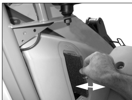
Fig. 183: Replacing the dust filter of the heating system
