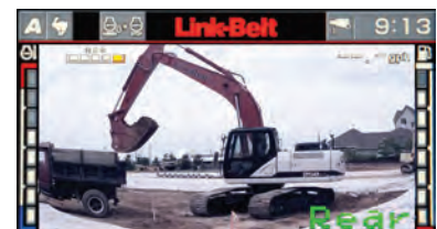
A standard rear-view camera displays a panoramic view of the worksite from the rear of the machine, an optional side-view camera is available.
