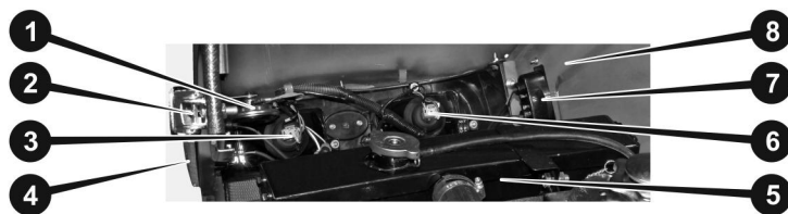
Figure 3.7. Front lighting and alarm devices
